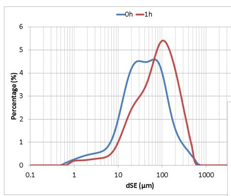
**dSE** = diameter of sphere equivalent.
