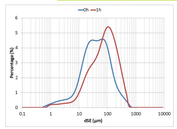
**dSE** = diameter of sphere equivalent.
