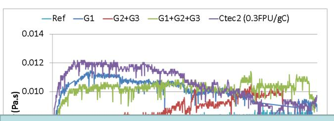
Sugarcane bagasse 30gdm/L Mixing rate 100rpm Ref: no enzyme **G2+G3** (exo-glucanase & βglucosidase) = small contribution.
