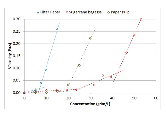
**Viscosity** at 100 rpm of SCB, FP and PP suspensions in relation with **biomass concentration**
