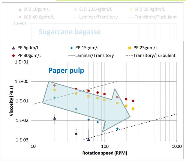
Suspension viscosity at different mixing rate
