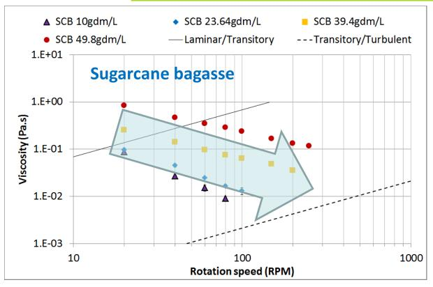
Suspension viscosity at different mixing rate
