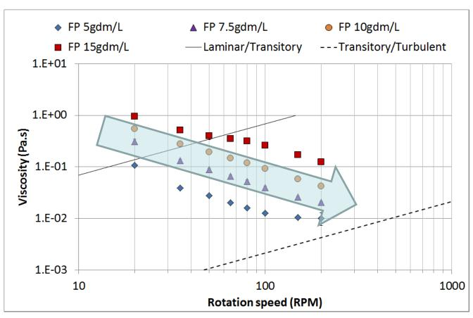
Suspension viscosity at different mixing rate
