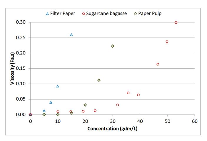
**Viscosity** at 100 rpm of SCB, FP and PP suspensions in relation with **biomass concentration**
