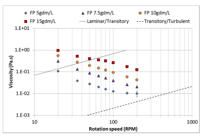
Suspension viscosity at different mixing rate
